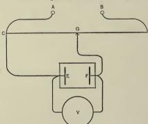
primary batteries, secondary batteries, dynamo or lighting circuit. The electrolytic cell is connected so that one pole E connects with C and the other pole F connects with the movable point or slider G so that any point of the conductor CD can be selected and any voltage from zero (when G is at C) to the full
